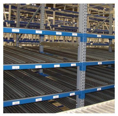
Ideal carton stock rotation system for applications with numerous SKUs. Flow options are available to handle full cartons, split cases, or piece picking. Carton flow can be configured in many different ways; as stand-alone, integrated with various pallet rack types, or within a multi level pick module.
