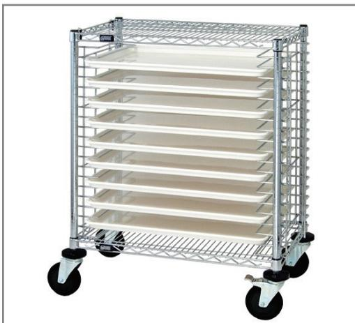
Tray carts are offered in half size and full size units, designed to handle work in process. Trays can be used on tray cart for conductive applications with the addition of aluminum split sleeves and a drag chain. Tray stop can be added to retain trays during transporting. All trays are manufactured of fiberglass reinforced thermoset material and can withstand temperatures of -40° to 250°F.
