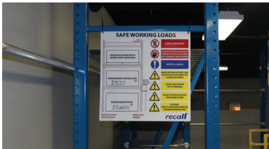
Display safe working loads for each level of racking when possible.
