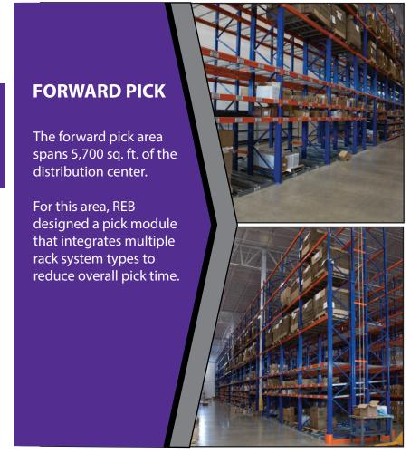
The pick module is also designed to accommodate a catwalk level to allow for future vertical expansion.
