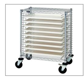
Tray carts are offered in half size and full size units, designed to handle work in process. Trays can be used on tray cart for conductive applications with the addition of aluminum split sleeves and a drag chain. Tray stop can be added to retain trays during transporting. All trays are manufactured of fiberglass reinforced thermoset material and can withstand temperatures of -40° to 250°F.
