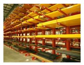
Cantilever rack is ideal for long or bulky items such as lumber, furniture, and plumbing because the system allows for easy product accessibility for heavy and lengthy items.
