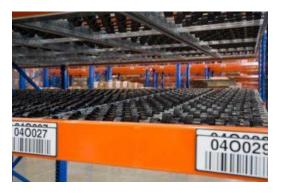
Rack supports inclined rollers or wheels that allow cartons to glide from the back (loading) aisle to the front (picking) aisle. Brakes can be included for speed control. These gravity systems provide excellent volume utilization. Carton flow can be configured in many different ways, such as a stand-alone system, integrated with various pallet rack types, or within a multi-level pick module.
