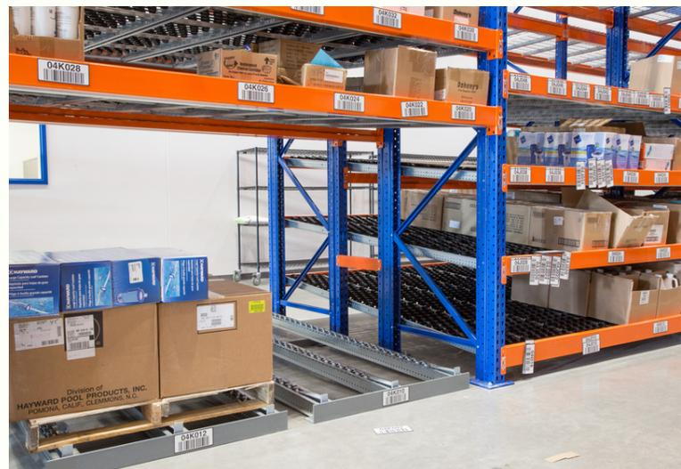
In this example, two-deep pallet flow was included on the ground level for faster-moving products. Two levels of carton flow were integrated with the pallet flow for case picking of items that need replenishment closer to the 1-month range. Five levels of selective rack were included on top for the immediate product replenishment of the carton and pallet flow.
