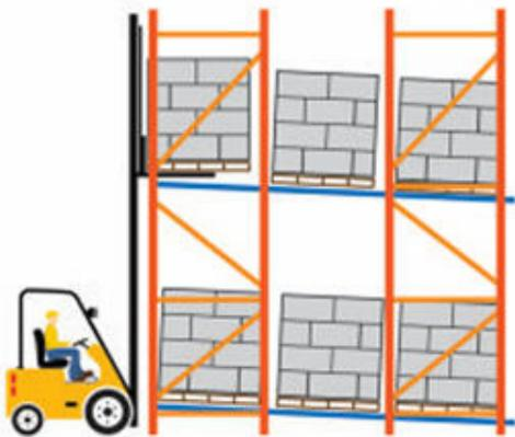
*Pallets are loaded from the back of the system and glide to the front for picking. When the front pallet is unloaded, the next automatically glides into picking position.*
