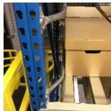
**Kickplates:** Can be Implemented to prevent personnel traveling on the upper levels from tripping by eliminating space along aisles and row ends. Kick plates are recommended to be installed on the upper levels of the system at all aisle row ends and along all main aisles.
