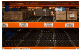
Carton flow rack is made up of uprights, beams, and inclined lanes of rollers or wheels that allow cartons to glide from the back loading aisle to the front picking aisle. When the front carton is unloaded, the next automatically glides into picking position.
